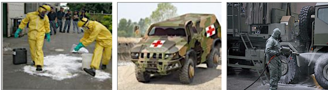
Figure 2.1. Represents the use of BX24: (a) as an Active Sorbent of a hazard spill (b) as Sol-gel - Preventive sacrificial/ self-decontaminating coating (c) as liquid Post-event decontamination, according to NATO Levels of Active Decontamination Operations.
