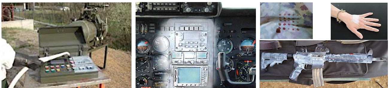
Figure 2.4. Removal of contaminant by vacuuming SX34's dried formula off electronic equipment, SX34 applied to fix and absorb contamination of flight instruments, military uniform, skin, and a personal weapon, prior to removal of the absorbed and dried contaminant.
