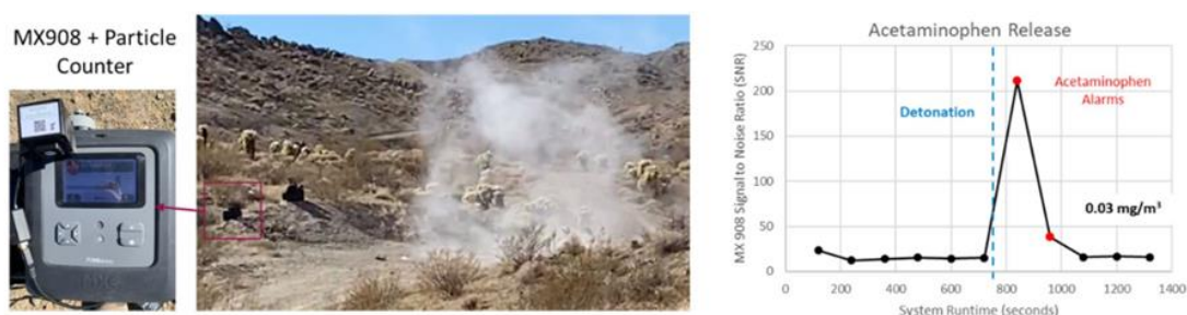
Figure 3.3: Aerosol module field testing. Left to Right – An MX908 outfitted with an Aero and co-located with a particle counter to provide ground truth measurements of the aerosol plume. Overview image an acetaminophen aerosol plume formed from a recent detonation. MX908 system response before, during, and after detecting the acetaminophen aerosol plume. Plume concentration detected at the MX908 was 0.03 mg/m 3 .
