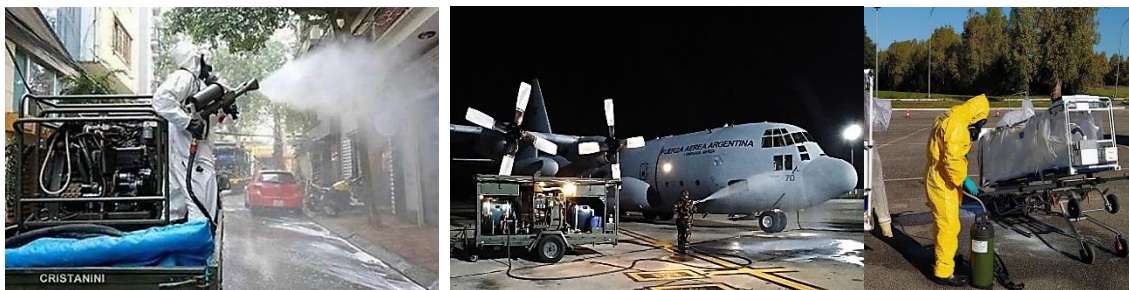
Figure 2.2. BX24 sanitisation against COVID-19 (a) in urban environment mode (b) sanitation of the exterior of aircraft and (c) a Stretcher Transit Isolator.
