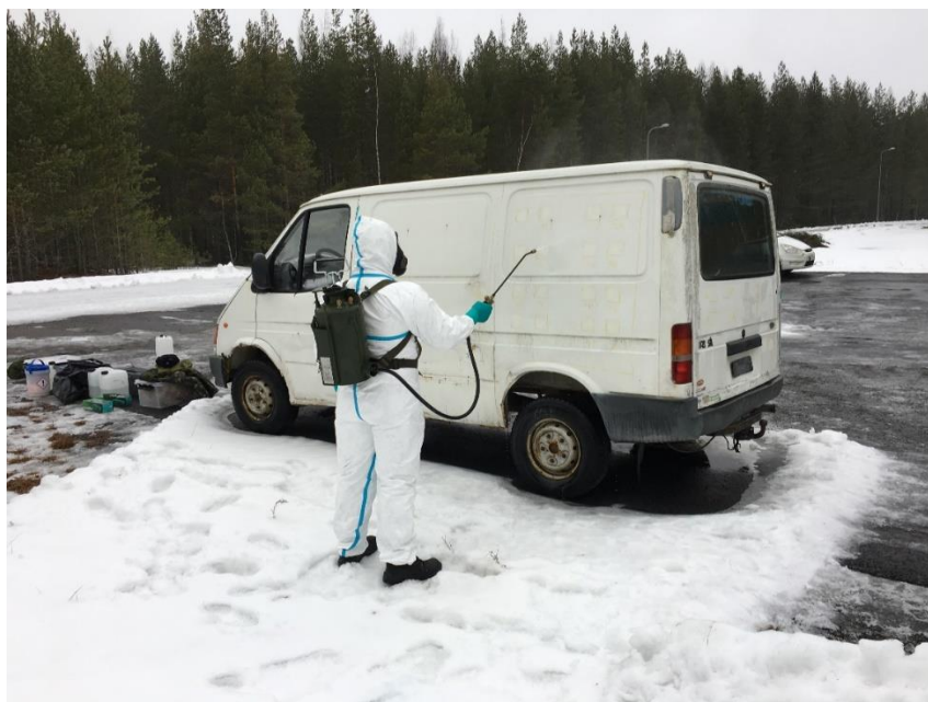
Figure 4.1: The first test of first field study: a van contaminated with a chemical warfare agent simulant DEA.
